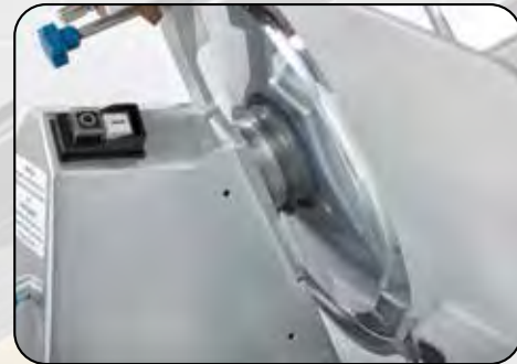
Switches mounted on top to reduce failures
